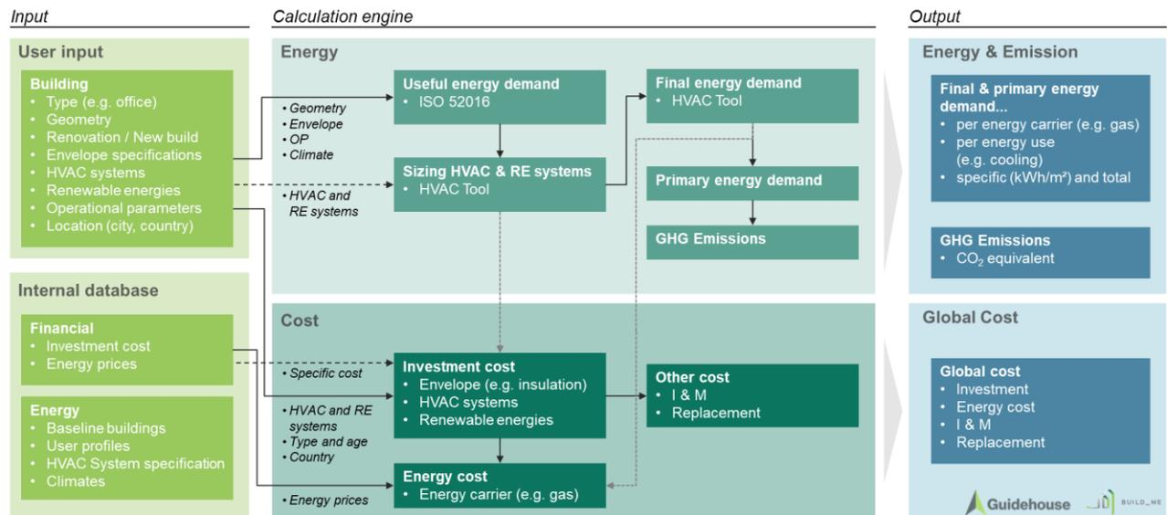
Figure 3. BEP Tool calculation procedure
